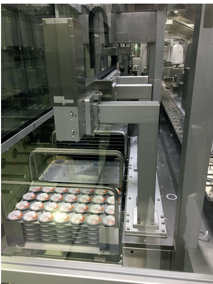
Fig. 1. The inhalers are fully automatically mounted in the cleanroom (© Witosa)
